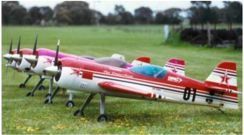
Damien Mould, Giles Hill, Damien Milk and Stephen Green's 1/3rd scale Sukhoi SU 26. Wingspan 2.3 metres- weight 12.5 kg power Zenoah 74cc twin cylinder two stroke. Yarra Glen Sept 1996.
