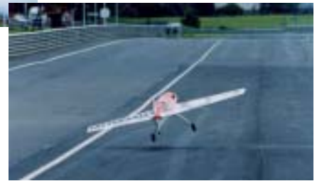
The rudder pitch coupling made it a pig landing crosswind. I hated bouncing it but the crowd didn't..
